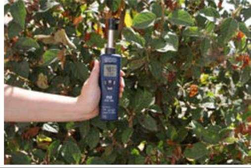
With the PCE-555 hydrometer you can measure ambient conditions including humidity in the top portion of the LCD and temperature shown on the bottom and also calculates wet bulb temperature and dew point, which are useful for calculating thermal stress.
